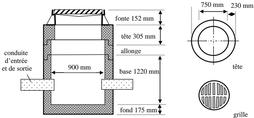
ILLUSTRATION 4.3 PROFIL D'UN PUISARD DE POLYÉTHYLÈNE OU D'ACIER ONDULÉ
